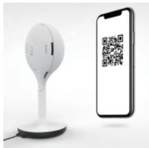
Please point the QR code in the screen of the mobile phone towards the device and keep the distance of about 15~25cm. Wait for the device to scan the QR code on the mobile phone.
